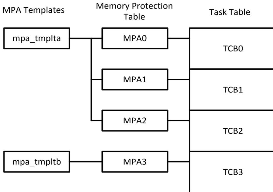
To the left of TT is the Memory Protection Table (MPT). This table has a Memory Protection Array (MPA) for each task. MPAs are in the same order as TCBs, and each TCB contains an index into MPT to access its MPA. A task's MPA is loaded into the MPU when the task is dispatched. Thus, each task has its own set of regions when it is running. The overhead on task switching time is about 25% for an MPA with 5 regions.
